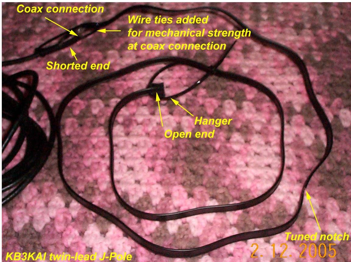
In an emergency situation, it is often necessary to squeeze every bit of performance possible out of a 2 meter HT. One way to do that is to replace that little rubber duck antenna with the ever-popular Twinlead J-Pole. This simple antenna lends itself well to emergency use or as a portable antenna for hotel room operations while traveling.
