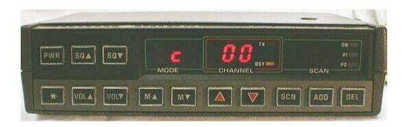
Once all the changes are made tap the squelch (SQ) up key to write the data and reset, it will reset and return to normal operation. Set the switch back to normal for operation.
