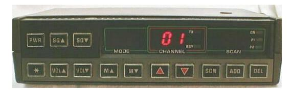
Again tap the "\*" key. This gets you to the transmit frequency, the TX light will be on to indicate this, but the radio is not transmitting so don't worry! Use the mode, channel and scan keys to change the data:
