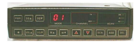
Once the MODE is selected, tap the "\*" key, This will now move you to the CHANNEL window to select which channel you will modify. The channel up and down buttons are used:
